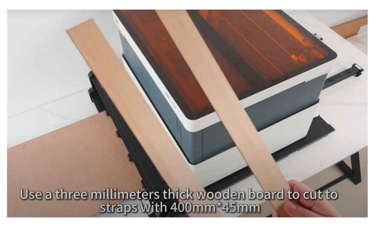
4. Before starting a task, we recommend clicking the **Framing** button in the preview window to observe the laser head's movement path and confirm that the material's length and flatness are appropriate. This helps prevent issues such as material jams or insufficient material length during the entire processing. Normally we suggest the materials should be 50cm longer than your design.
