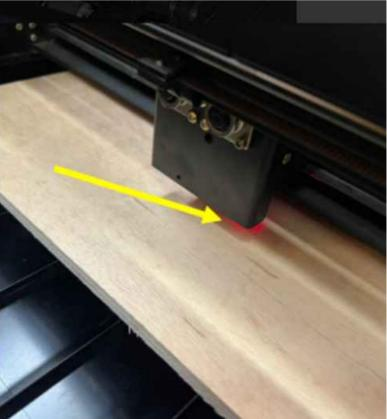
6. In cutting mode, it is advisable to enable the **Breakpoint** feature to prevent small cut pieces from dropping and potentially causing material jams during work. Remember to add the number of breakpoints according to the size of the cutting area. Here is guidance about using breakpoint: https://support.wecreat.com/hc/en-us/articles/9081665785103-Parameters-Setting
